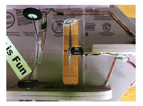
Bend the gear so wheel cc ar 9.5" and height is 5.5"
