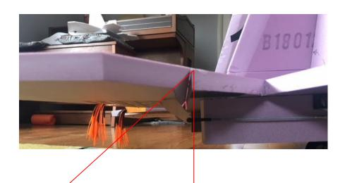
Cut out 45 deg angle in elevator
